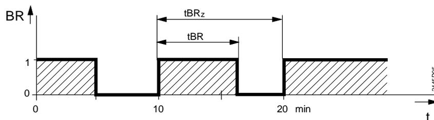
$$q = \frac{t_{BR}}{t_{BRz}} = \frac{6 \text{ Min.}}{10 \text{ Min.}} = 0,6 \text{ (60 \%)}$$
